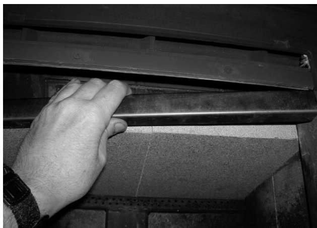
Figure 16 - Removing/Replacing the Baffle for Inspection
