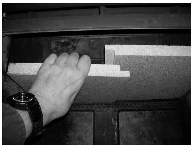
Figure 16 - Removing/Replacing the Baffle for Inspection
