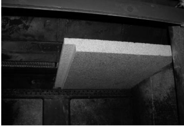
Figure 16 (cont.) - Removing/Replacing the Baffle for Inspection
