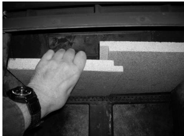
Figure 16 - Removing/Replacing the Baffle for Inspection
