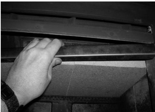
Figure 16 - Removing/Replacing the Baffle for Inspection
